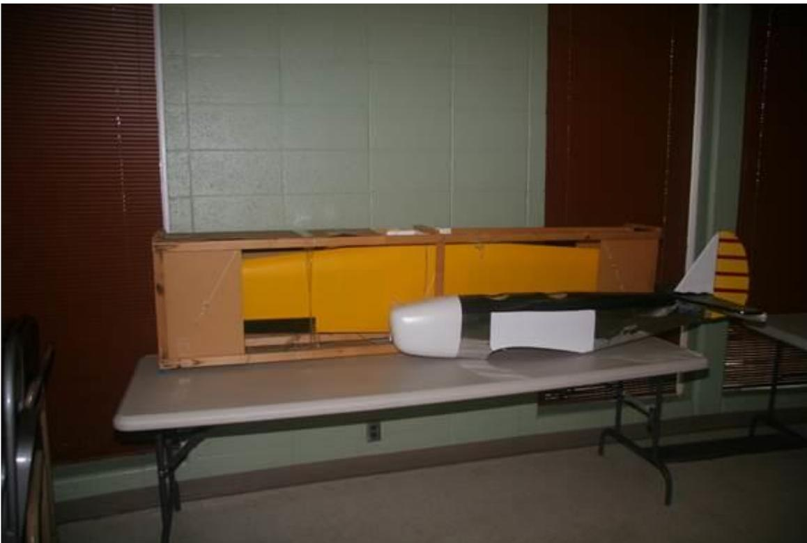
This picture shows the Fuselage with cowl and crated wing. There is also a box of components not shown.
