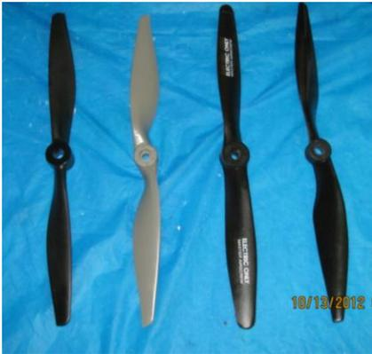
Apprentice 15e. The Apprentice's stock propeller is an E-flite 11x8 (EFLP11080E). I ordered several Apprentice propellers but out of curiosity I ordered three similar propellers from three other brands and tested each on the Apprentice for possible over-amping of the stock electronic speed control (ESC) and 15e motor. The test subjects are shown in the photo. From left to right the propellers are E-flite 11x8 electric, APC 11x8 electric, Master Airscrew 11X7electric, and Great
