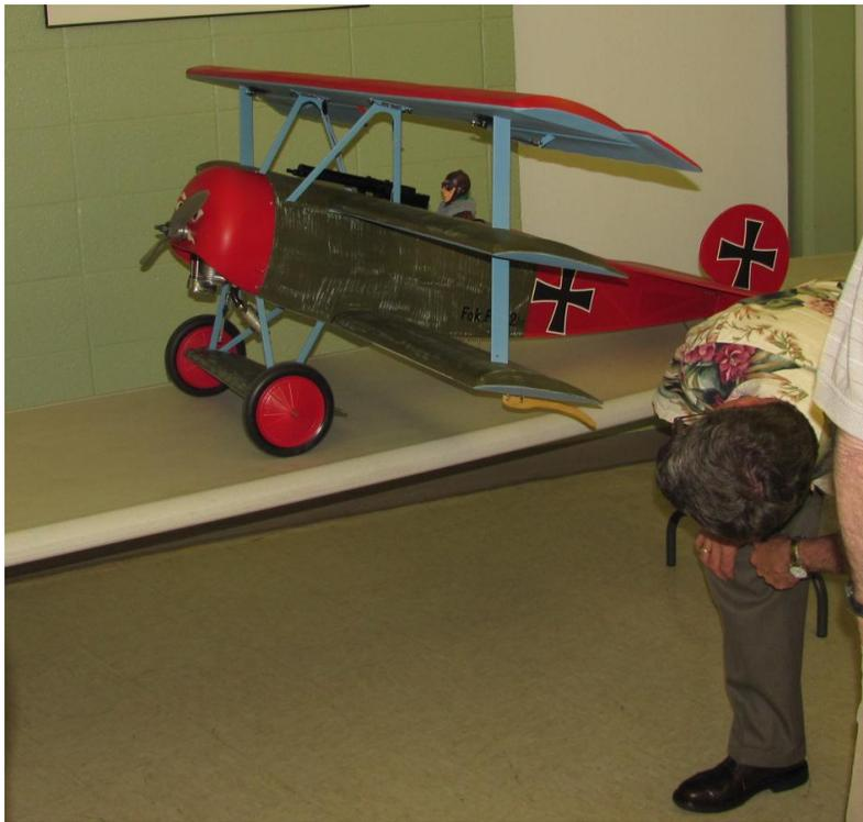
In the photo to the left is the Tri-wing aircraft which won Model of the Month in August for builder/pilot Rick Hunter. This Fokker DR-1 model required many hours to build such that construction required a year of work. Notice the skid-like devices under the lower wing. Apparently these airplanes have some ground handling issues which result in damaged wingtips. The skids are referred to as "axe handles" and prevent lower
